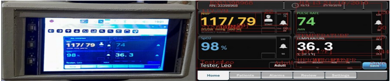
Figure 2: Optical Character Recognition (OCR) capturing image from the Vital signs monitor screen
